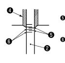
Marker line for DP x 17 needle (with needle count higher than #22)
