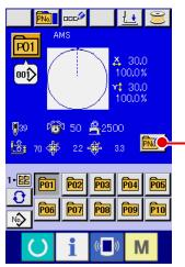
In case of the pattern button, 2-step stroke position can be set to each pattern button data.
