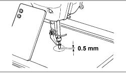
Setting range of the intermediate presser is up to the standard of 3.5 mm. However, the setting range can be changed up to max. 7 mm with memory switch U112.
