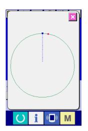
When VIEWER button *(K)* is pressed, the shape of the pattern No. selected is displayed and you can confirm it.
