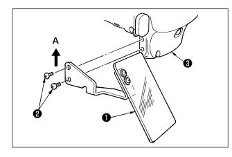
Use eye protection cover **1** after securely attaching it on face plate cover 3 with screw 2.
