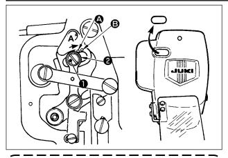
By removing the rubber plug in the face plate cover, adjustment can be performed without removing the face plate cover.
