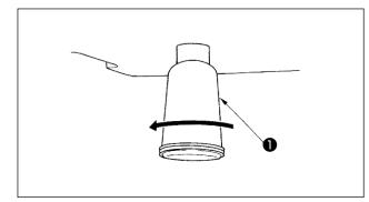
When polyethylene oiler **1** becomes filled with oil, remove polyethylene oiler **1** and drain the oil.
