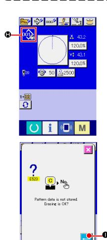
When X/Y enlargement/reduction ratio, thread tension, intermediate presser, adding/deleting of thread tension command, or adding/ deleting of increase/decrease value of intermediate presser of users' pattern or media pattern is performed, the pattern kind section becomes change display **①**.
