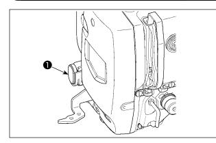
When TEMPORARY STOP switch **①** is pressed during sewing, the sewing machine can be stopped. At this time, the error screen is displayed to inform that the stop switch has been pressed.
