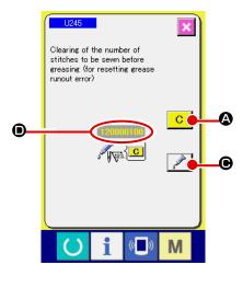
When the sewing machine has been used for a certain number of stitches, error "E220 Grease-up warning" is displayed. This display informs the operator of the time of replenishing the designated places with grease. Be sure to replenish the places with the grease below. Then call the memory switch U245, press CLEAR button
