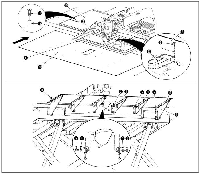
1) Move the cloth feed base to the rear and place throat plate auxiliary cover (asm.) ③ from between lower plate ① and throat plate ②.
