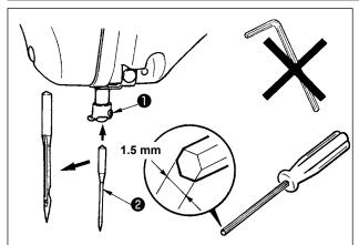
Loosen setscrew **①** and hold needle **②** with the long groove facing toward you. Then fully insert it into the hole in the needle bar, and tighten setscrew **①**.
