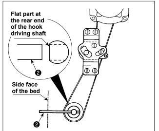
2) Face the flap section of the rear end of hook driving shaft to the frame side, and insert hook driving shaft positioning shaft (2) (13704705) supplied with the machine as accessories from the hole on the machine bed side.
